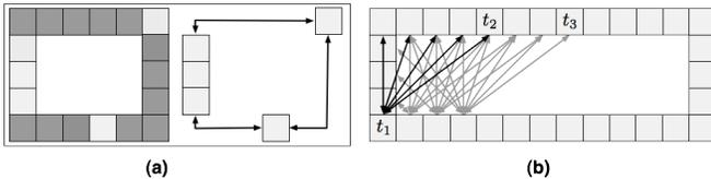
Figure 2: (a) We prune all (dark grey) nodes which have no neighbours in any adjacent rectangle (left). Remaining nodes (right) are then connected directly. (b) Assume  $t_1$  is the parent of  $t_2$ . When  $t_2$  is expanded, we do not generate neighbors from the opposite side. These can be reached from  $t_1$  via a shorter or equal-length path.
