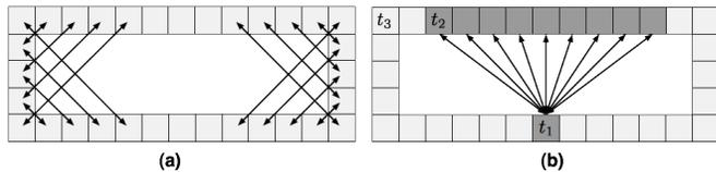
Figure 1: (a) Macro edges between nodes on orthogonal sides of an empty rectangle. (b) Each node on the perimeter is connected to a set of nodes on the opposite side.
